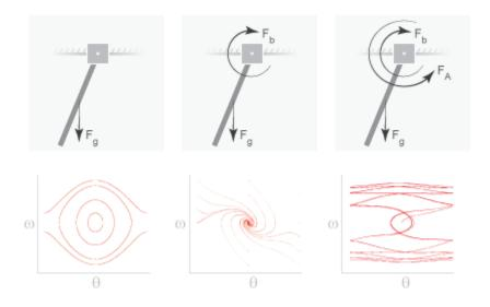
Your starting point is the simple pendulum model that you built in "Model a Simple Pendulum" on page 1-19. By adding forces and torques to this model, you incrementally change the pendulum from undamped and free to damped and driven. The forces and torques that you apply include:
