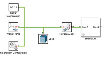
**6** In the Solid block dialog box, specify the following parameters. This block connects rigidly to the World frame and therefore has no effect on model dynamics. You can leave the inertia parameters in their default values.
