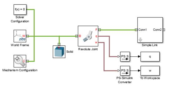
Joint block port q, and that the To Workspace block with variable name w connects to the Revolute Joint block port w.
