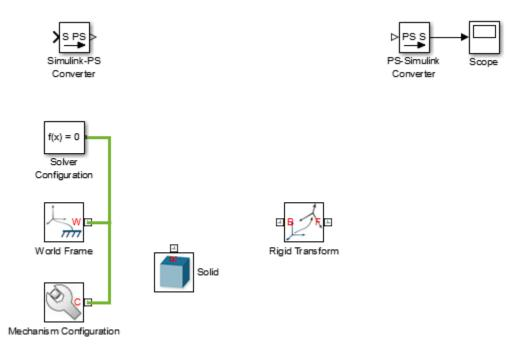
You can also open the Simscape Multibody block library from the MATLAB command prompt by entering sm\_lib. Browse the library to select blocks for your model. Alternatively, type the block name in the Simulink Model window and select a match from the Simulink search results.
